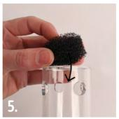
Replace the sponge back in the centre media chamber and then replace the lid, ensuring the seal is correctly positioned within its groove.
