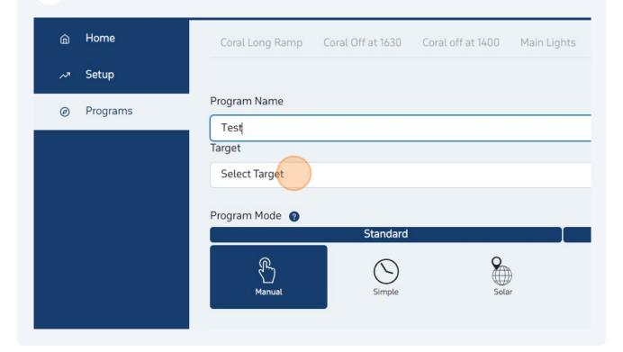
Create your Program. 'Manual' sets a permanent lighting level. 'Simple' allows for an on/off ramp photoperiod. 'Solar' will vary the length of photoperiod based on an entered geographical location. The 'Drift' modes allow for a transition from one program to another over a set number of days. 'Custom' requires a user dataset, creating any possible required photoperiod.
