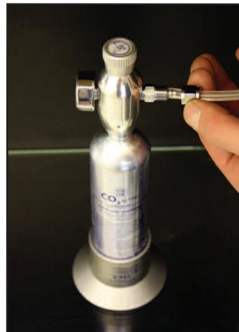
At a convenient position between the pressure regulator and the bubble counter make a cut in the flexible tubing and install the non return valve.
